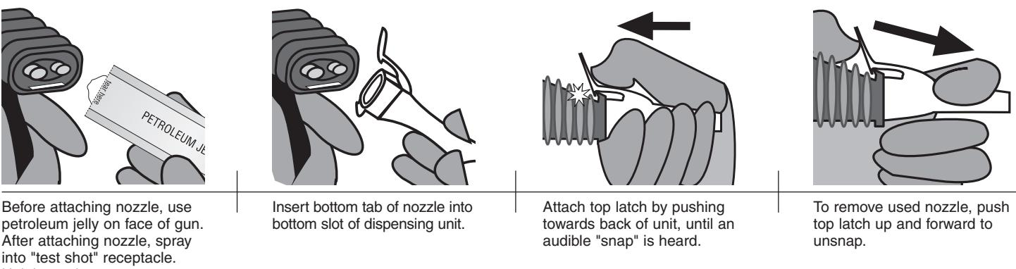
Before attaching nozzle, use petroleum jelly on face of gun. After attaching nozzle, spray into "test shot" receptacle. Unit is ready to use.
