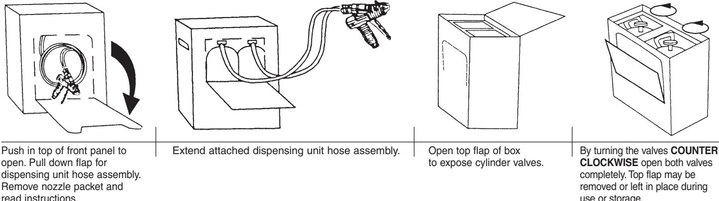
Push in top of front panel to open. Pull down flap for dispensing unit hose assembly. Remove nozzle packet and read instructions.
