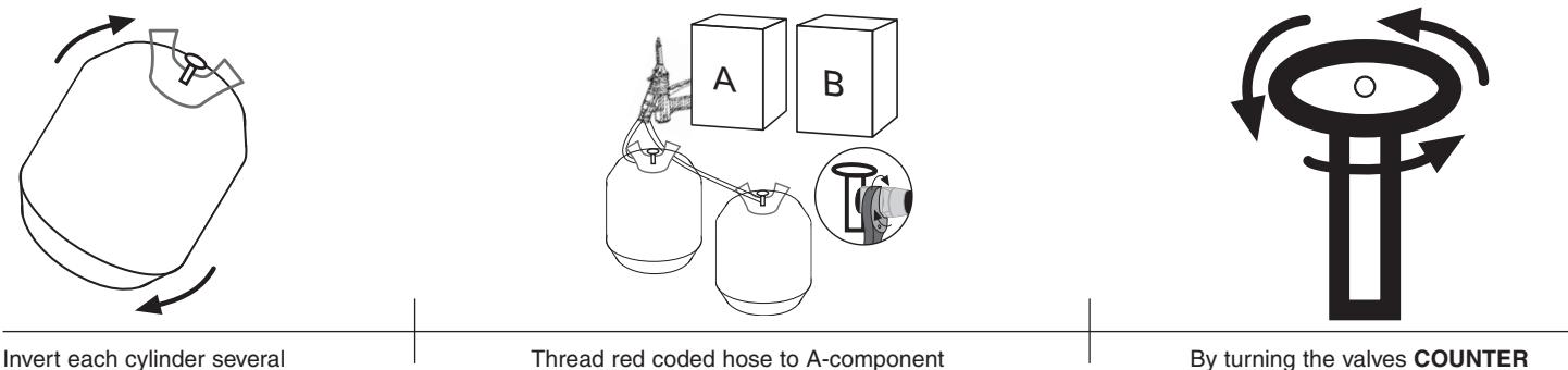
Invert each cylinder several times before use to insure proper mixing.
